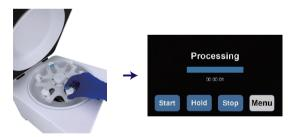
Note: When the processor runs for more than 0.5 hours, it is recommended to stop the operation and open the cover to dissipate heat for 15 minutes, as the temperature of the processor will fise to more than 185°F (65°C) after continuous operation for more than 1 hour.
